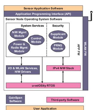
system solution for Wi-Fi sensors based on GainSpan's GS1010 SoC.
