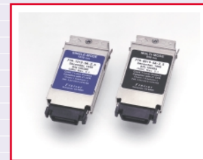
Finisar 2.5 Gbit/s rated Instrument Grade GBICs insure high signal integrity.
