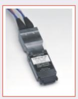
Finisar 2.5 Gbit/s rated Snoop GBICs provide a totally transparent attachment to the system under test.
