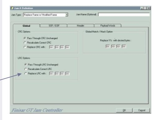
The FICON Jammer has the added ability to pass the LRC unchanged, recalculate the correct LRC, or replace the LRC with a ser-defined value.
