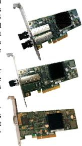
The transition to SFP+ modules allows the Chelsio adapters to be used either with twin-ax copper cable or with fiber cable, as well as enabling a price reduction across the product line. All of the new 10GbE adapters are available today directly from Chelsio and its distributors.
